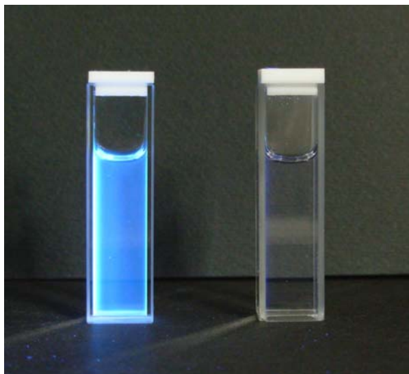
Figure 8. Photo of the sample of L1 in \text{CH}_3\text{CN} solution: alone (right) and in [\text{OH}^-] = 1 \times 10^{-2} \text{ M} (left).
